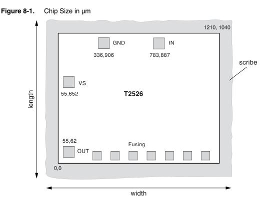
Note: Pad coordinates are given for lower left corner of the pad in  $\mu$ m from the origin 0,0
